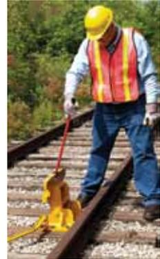
**Use Aldon® Derail Lifting Lever** to reduce the lifting effort by 60%
