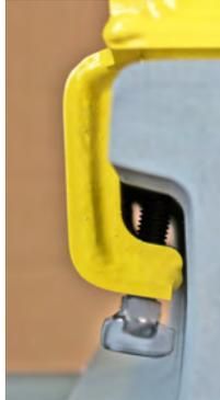
6. Tighten locking arm screw and then tighten all three screws on field side. **All four screws must be tight. Derail must be level and straight.**
