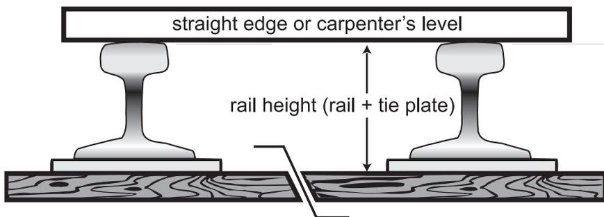
**NOTE:** make sure there is no gap between rail, tie plate, and tie. Any such “daylight” must be removed by lifting the tie and re-tamping
