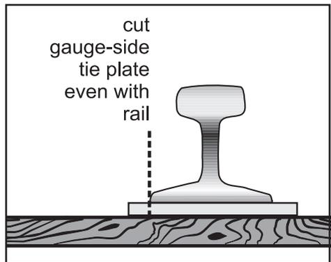
**Never leave any gap between the rail and tie.** Any such gap will create an insecure foundation for the derail.
