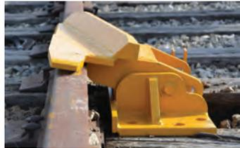
**Too Low.** A derail block that does not lie flat will cause a failure to derail.
