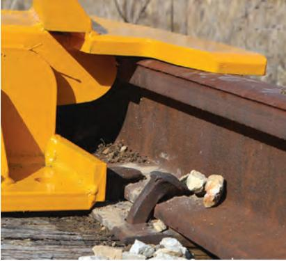
The derail sits on two ties and must be pushed up against the rail head. The tie plates inside the rail will get in the way, so it is necessary to crop the plates close to the base of the rail. The derail base must sit flat on the ties.
