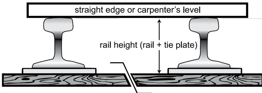
CAUTION: some derail installations will require shimming up the derail to equal height of rail. Shims should be steel plate, equal in size to the derail base flange, and through-bolted in order to properly secure the derail to ties. Make-shift shims do not provide a solid foundation.
