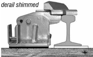
note that "height of rail" includes tie plate thickness
