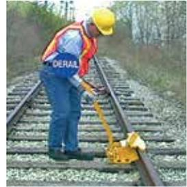
Always lower and raise the derail when you remove or reinstall the derail block.
