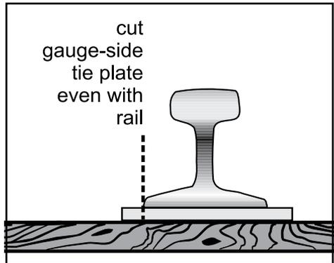
**Never leave any gap between the rail and tie.** Any such gap will
